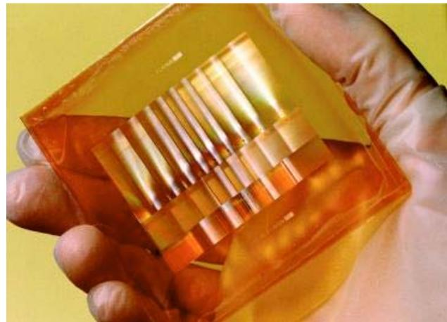
Fig. 1. Lenslet array recorded in photoresist for custom IR detector application.
